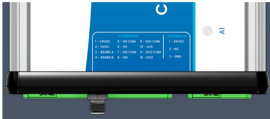
Figure 4 : Pinout of the J2 connector on the CAL-WIRELESS-BOX
