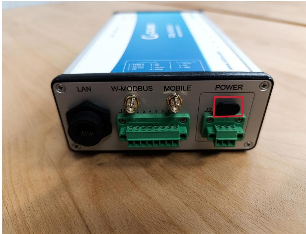
2. Remove the 4 screws on both sides of the device
