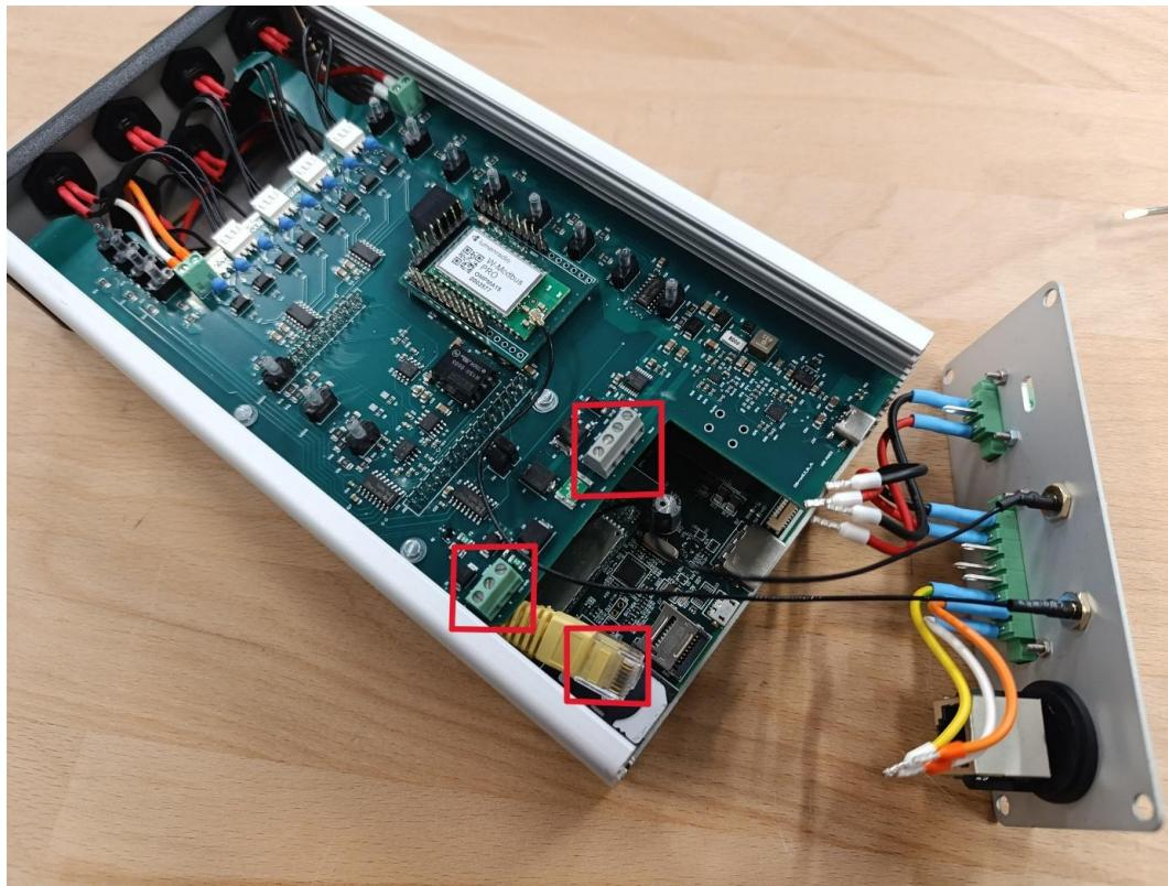
Unplug the cables from the two connectors and disconnect the UTP cable.
