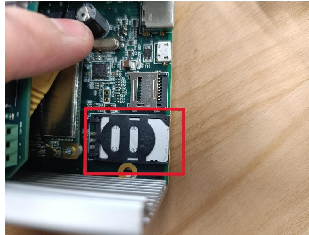
7. The location where the SIM card is located must be moved to the left to "unlock" it
