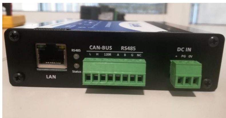
Figure 2 : Terminals on the CAL-EDGE-0 (front view)
