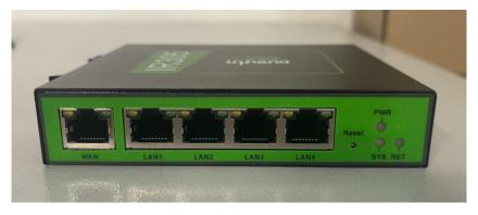
The CAL-EDGE-0 device should be connected to the port labeled LAN1.
