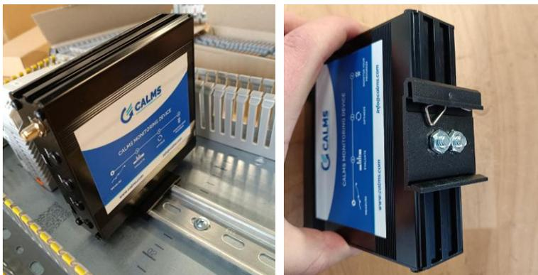
**3. Connectivity:** SIM card is already inserted. Connect Ethernet cable (if using a wired connection). Attach the antenna to the SMA connector.
