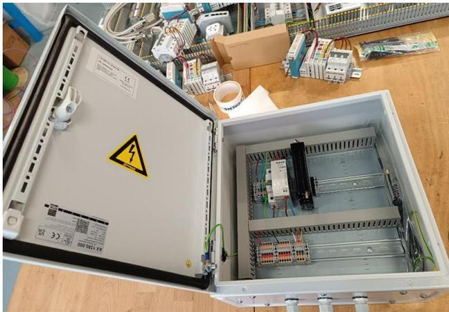
**2. Wiring:** Connect 230VAC supply to the internal power supply. Connect analog and digital sensors to the corresponding terminals. Use 4–20 mA sensors for AI and dry contacts for DI. Follow proper grounding: connect the mounting plate, cabinet door, and enclosure base to the ground terminal blocks.
