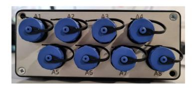
**A1-A8**: Analog sensors are connected to these connectors. Connectors are internally wired to 18bit resolution analog card.
