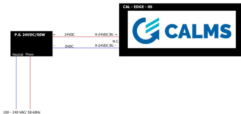
Figure 4: Power supply wiring scheme
