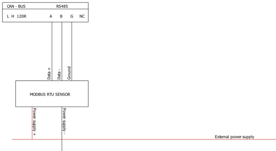
Figure 6: RS485 wiring scheme
